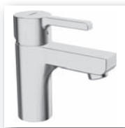
HANSAFORM one-hole single-lever basin mixer, DN 15 4905 2203 chrome without pop-up waste, connection with flexible hoses G 3/8 projection: 99 mm
